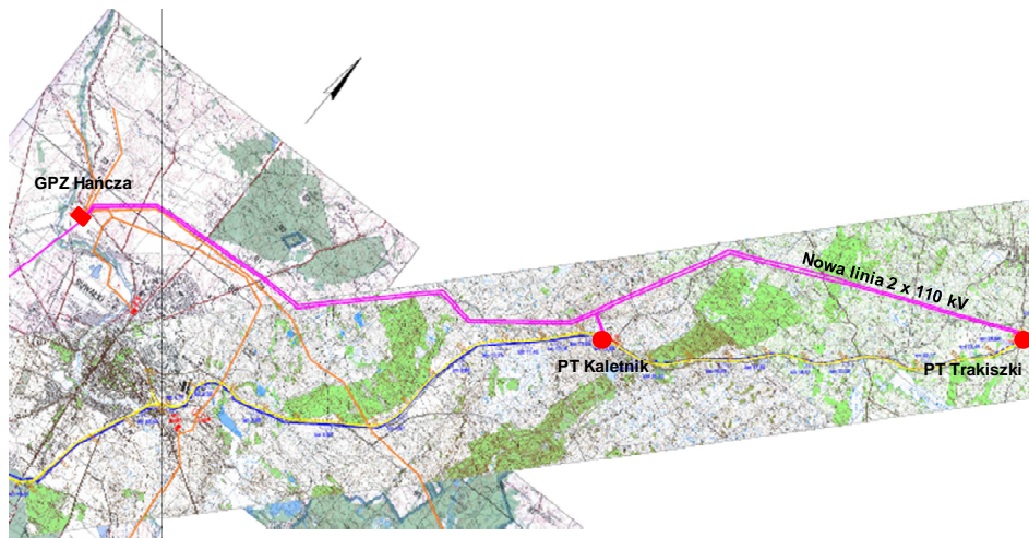
Fig. 2. Supplying of new traction substations on E75 line [4]
